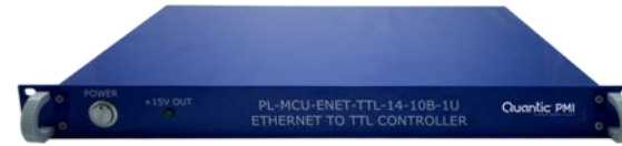
Ethernet Microcontroller Test Box
