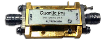
1 to 4 GHz, Voltage Variable Attenuator
