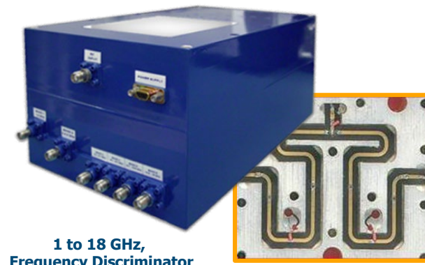
Delay Line in a Frequency Discriminator
