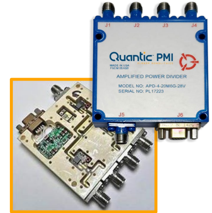
20 MHz to 6 GHz, Amplified 4-Way Power Divider
