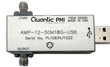
50 MHz to 18 GHz, 12 dB Gain USB Powered LNA
