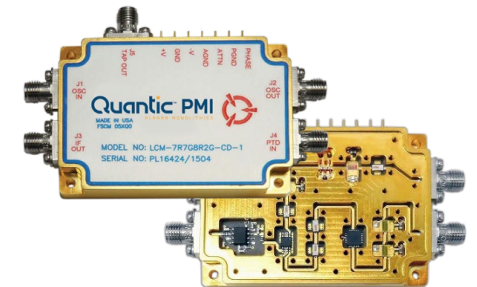
7.7 to 8.2 GHz Laser Control Module
