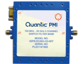
DC to 26 GHz 5-Channel Switch Filter Bank
