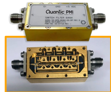
Miniature, 2 Channel Switch Filter Bank
