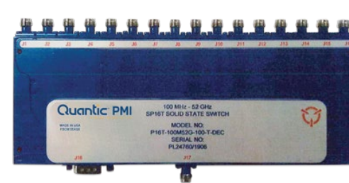
0.1 to 52 GHz SP16T Absorptive Switch
